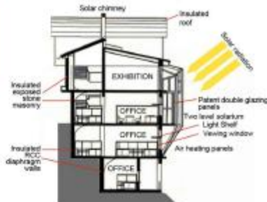
Section demonstrating various passive solar features integrated into the building envelope
